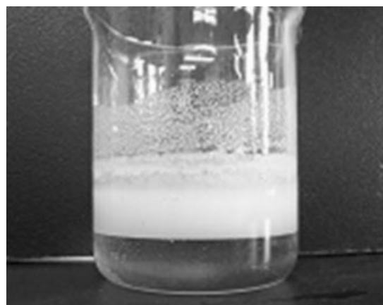
Figure 10 The delaminating of product after resting 20 min.
